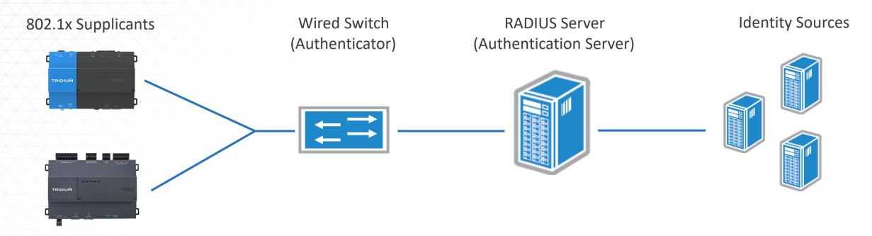
802.1x, an IEEE standard for network access authentication, is typically used in enterprises and campuses with large scale networks to provide security, scalability and ease of management. The JACE 8000 and Edge 10 are now compliant with this standard and can be used as wired clients (supplicants) in a 802.1x based network.
